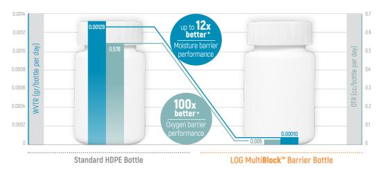
Oxygen Transmition Rate (OTR) - According to ASTM F-1307 23°C 50% RH ■ Water Vapor Transmition Rate (WVTR) - According to ASTM F-1249, ASTM E-96 38°C 90% RH
